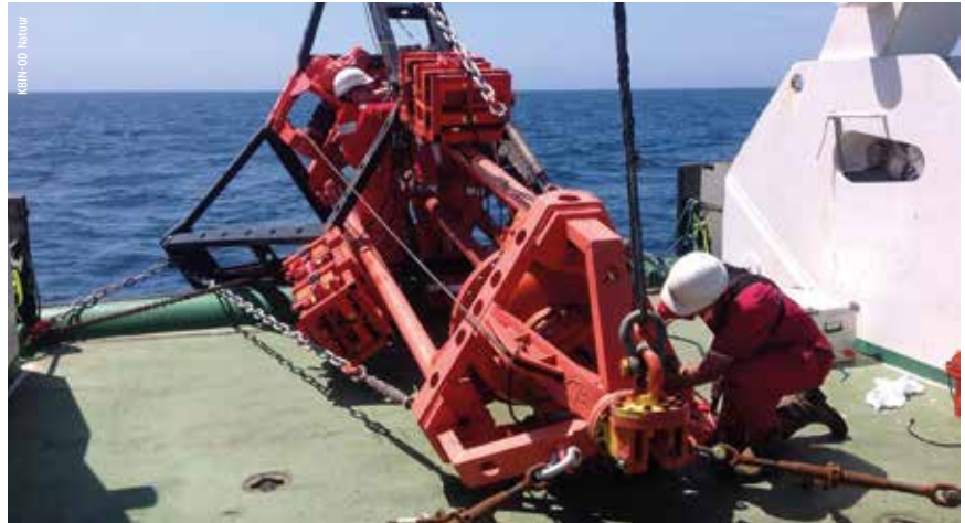
Scientists prepare their rock drill on the research vessel the Belgica to take soil samples
